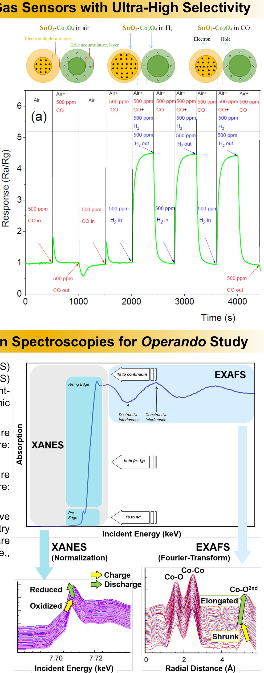
X-ray absorption fine structure (XAFS) and x-ray emission spectroscopy (XES) are techniques that probe the elementspecific atomic, chemical and electronic X-ray absorption near edge structure
